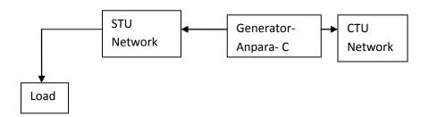
17. The power flow in such scenario depends upon the system conditions and is not in the control of the generator. As the STU network is feeding State load, all power of Anpara-C may be consumed by the State itself.
